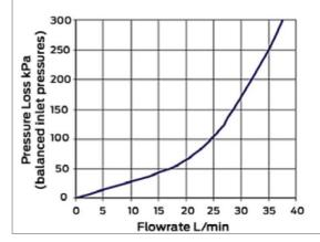
NOTE: To ensure optimum performance the minimum outlet flow of the TMV during operation should be at least 4 litres/minute.
