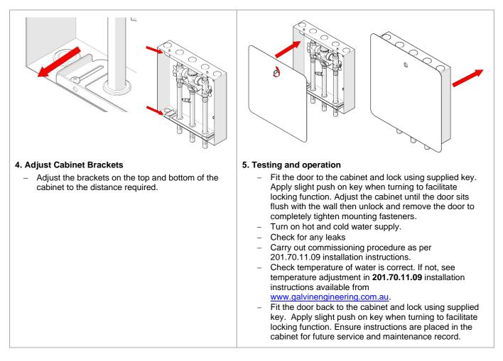
For commissioning, maintenance, temperature adjustment, spare parts and on-going servicing information refer to 201.70.11.09 Install from www.galvinengineering.com.au.
